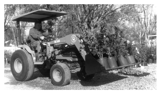
FILLING THE BUCKET Approach and enter the pile with a level bucket.
